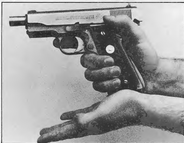
Phase One starts with the Tap: a weak-hand blow to the bottom of the magazine.
